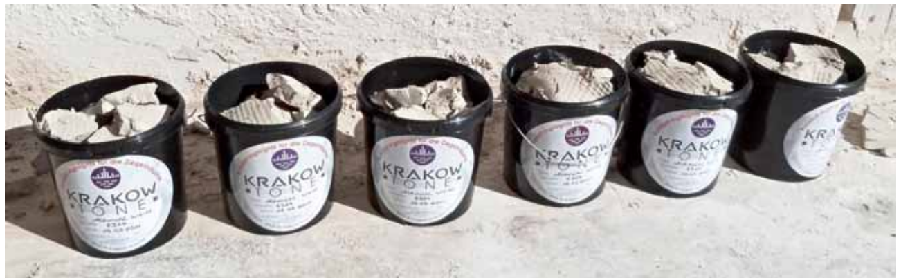
»3 Secondary raw material as a result of membrane filtration of marble sludge
