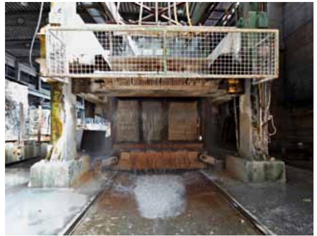
»2 Sawing of the marble blocks with the production of carbonate water suspension
