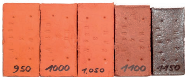
»6 Fired samples of the GS 6351 raw clay
